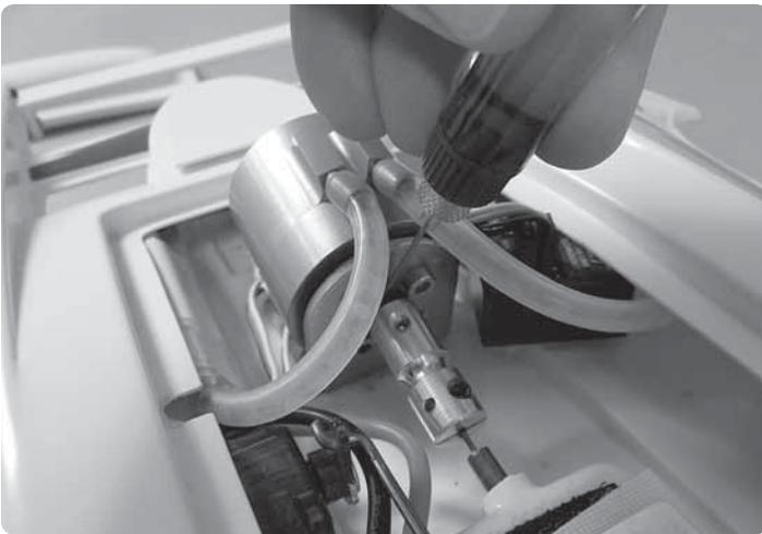
Remember to oil the motor bearings after each day of running. Just a few drops on each bearing are enough.
