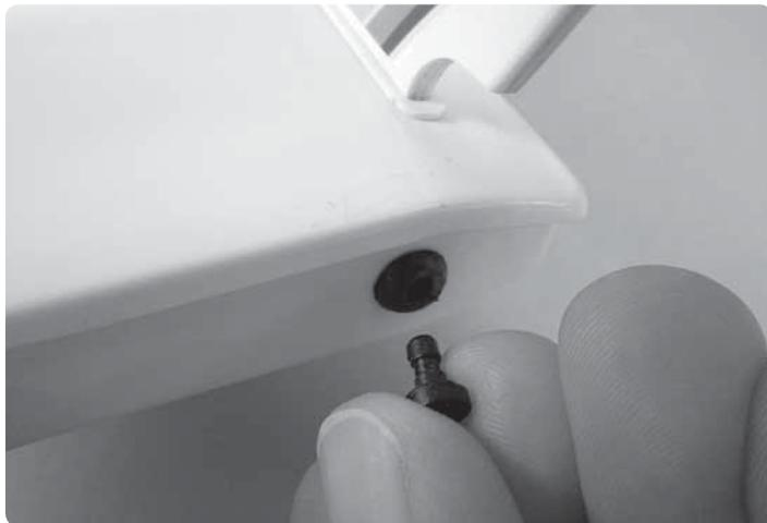
**IMPORTANT:** If your boat takes on a large amount of water and stalls, don't worry. **Foam flotation will keep it from sinking.** You will have to retrieve the boat and remove the canopy to release any water that might have entered. If the inside is flooded, remove the transom plug from the back of the boat and let the water drain. Allow the boat to fully dry before operating it again. Remember to re-install the transom plug before running.
