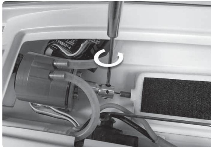
Using a 2mm hex wrench, loosen the screws holding the drive cable to the motor coupler. It is important to note that there are two set screws holding the shaft in position.
