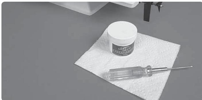
It is important to remove and re-lubricate the driveshaft after running for the day. Make sure the battery pack is unplugged. You will need a 2mm hex wrench, GrimRacer Cable Grease and some paper towels.
