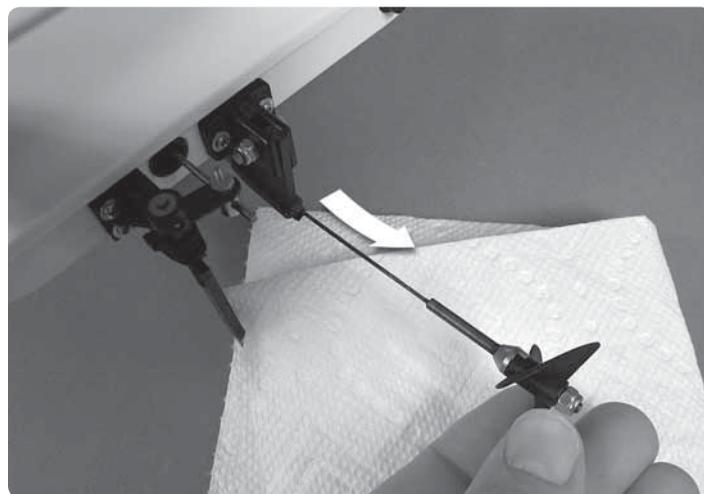
Slip the driveshaft out the back of the boat. Wipe off any grease and water that might be on the shaft. Using GrimRacer Speed Grease, apply a small amount to the shaft and slide it back into the boat. Be careful to align the driveshaft to the hole in the end of the motor coupler.
